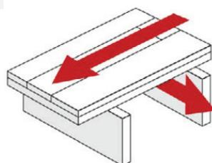
top and bottom layers together with construction adhesive and screw into the truss/ joist system every twelve inches. Additionally, nail (ring shank) or staple layers together on a minimum 12" grid pattern.
